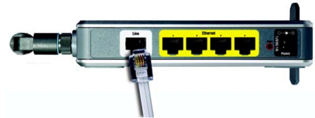
Figure 4-4: Connect the ADSL Line
